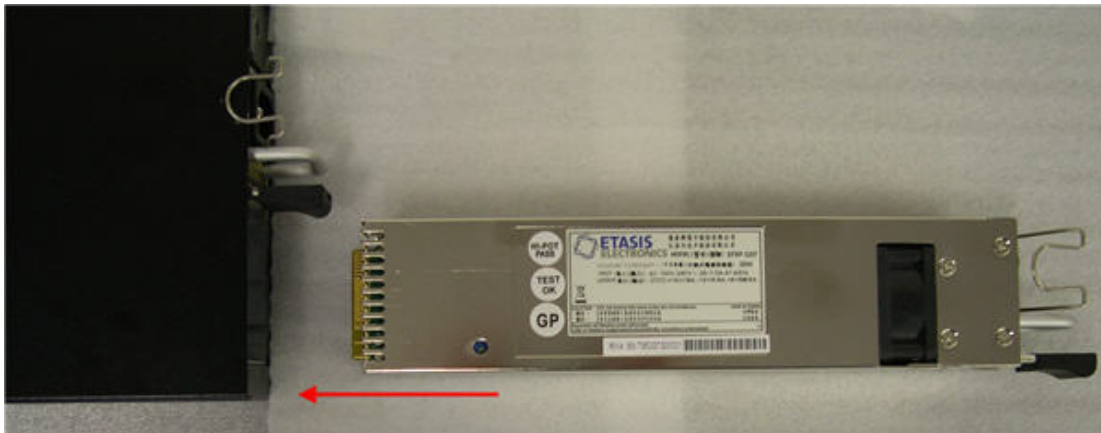
Figure 45 Slide the replacement power supply into the slot on the rear panel
